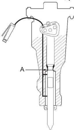
2. Lubricate the working tool's shank plentifully during all upward operations. The bushing and the working tool must be lubricated so frequently that dirt cannot penetrate into the hydraulic breaker.
