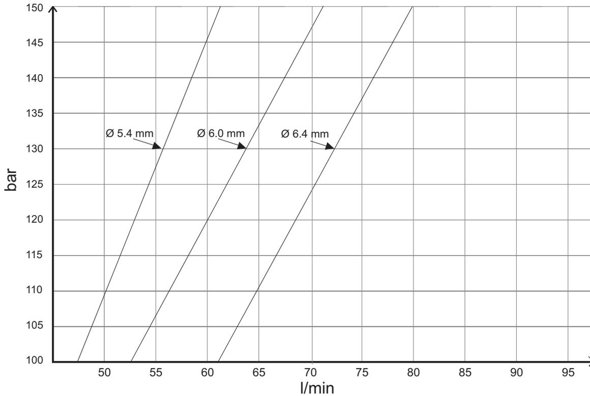
SB 302 Tunnel is delivered with restrictor Ø6.7 for 110 bar operation. As an option, restrictor Ø6.4 for operation at higher pressure, is available.
