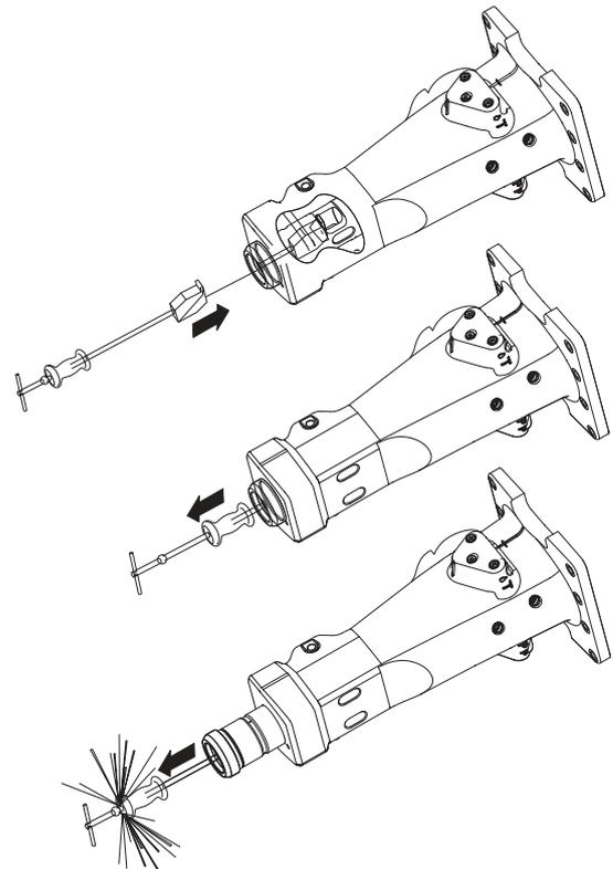
2. Carefully clean the bore and the bushing seat area.
